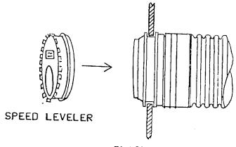
PLASTIC SEAL IN PLASTIC OR CONCRETE WALL
